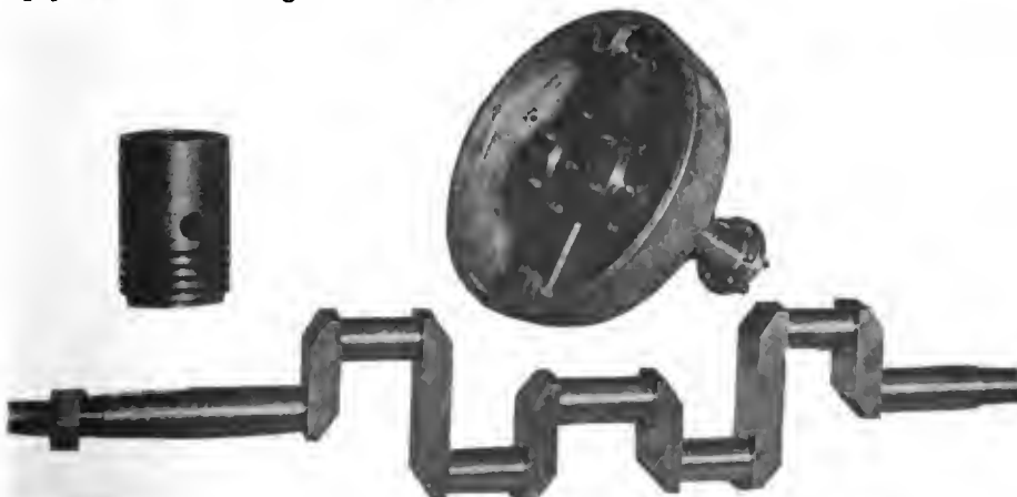
ALUMINUM CLUTCH, LONG PISTON AND FOUR-THROW CRANKSHAFT OF SIMPLEX CAR.
